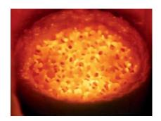
Breaking the coke habit: By coupling thermal decomposition with catalytic partial oxidation, an effective method has been developed to convert solid biomass such as cellulose into synthesis gas (see photo of a hot Rh catalyst surface). Not only is the process fast (<70 ms), it also avoids the formation of coke, which is known to deactivate catalyst surface sites and block surface reactions.
